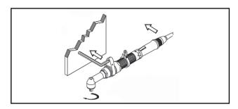
Fig. 7-1: Fixing the reaction bar
